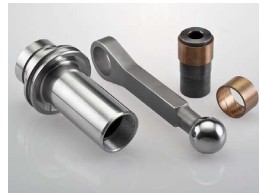
Suspension system damper; fatigue resistant steel, L1291 self-lubricating liner system, copper-based alloy bushings, 16" L when assembled.
