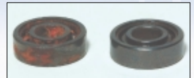
24-hour Salt Spray Test (Pat Chem Laboratories, Chrome Bearing and DLC Coated Chrome Bearing)
